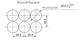
Note: above installation gap is the min value, please determine the installation hole gap according to equipment operation property and using property.
