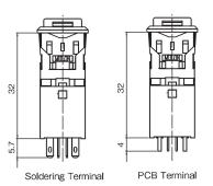
\* Switch Unit Terminal should be Soldering Type for both sockets.
