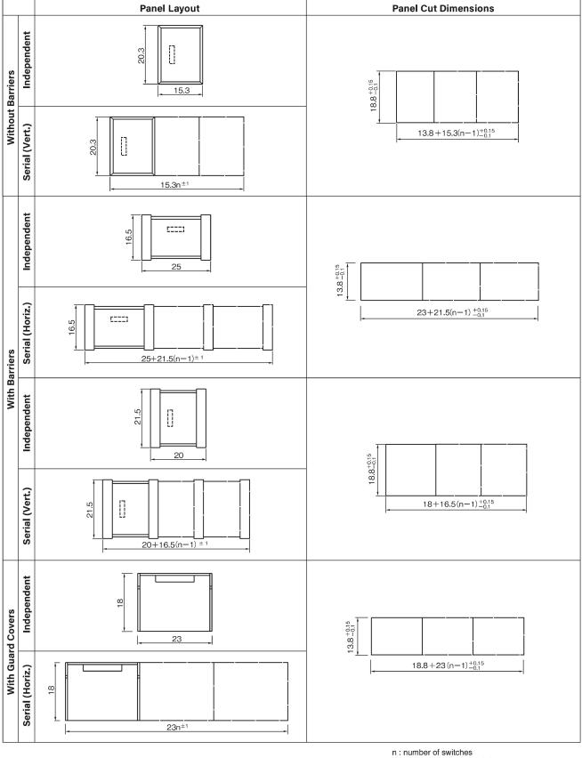
Panel thickness : 1mm~3.2mm Panel thickness for Guard Cover use : 1mm~2.5mm Tolerance : ±0.4mm
